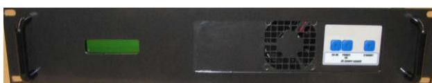
Meter shown mounted in a 19" sub rack with DC power supply unit
